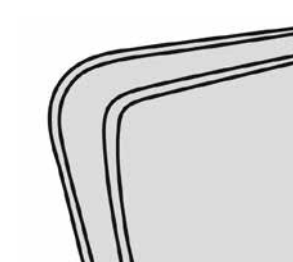
SBW = Small Box Border-2" with Welt LBW = Large Box Border-2½" with Welt
