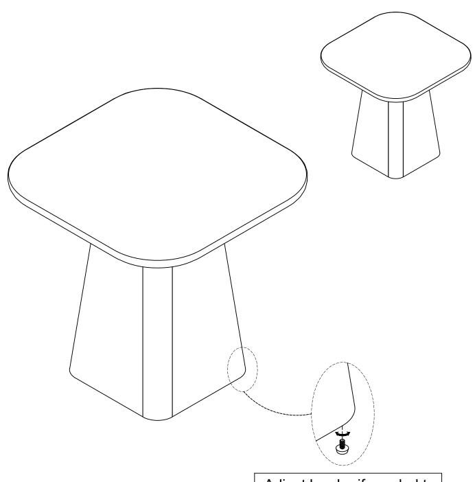
Adjust leveler if needed to level case on uneven floor
