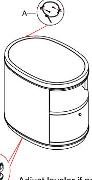
Adjust leveler if needed to level the table on uneven floor.
